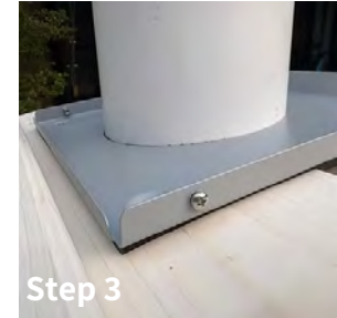
Step 3 Install external wall plate; the extension hood is recommended for thin walls (less than 240mm).
